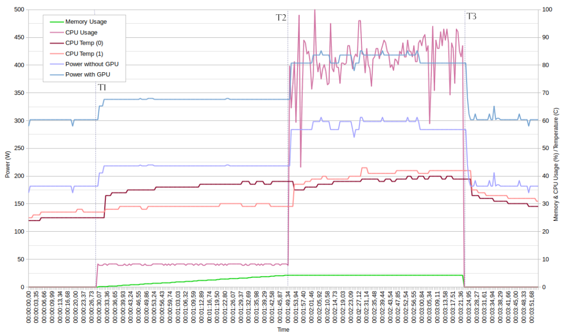
Figure 5: Results for the ComCiDis CPU collected by the IPMItool based monitoring application.
